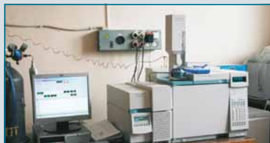
Chromatography-mass spectrometric system Agilent 6890N/5973N for identification of complex compounds
