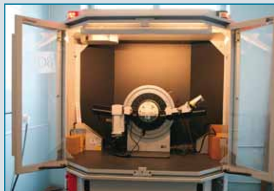
Diffractometer D8 ADVANCE BRUKER AXS
