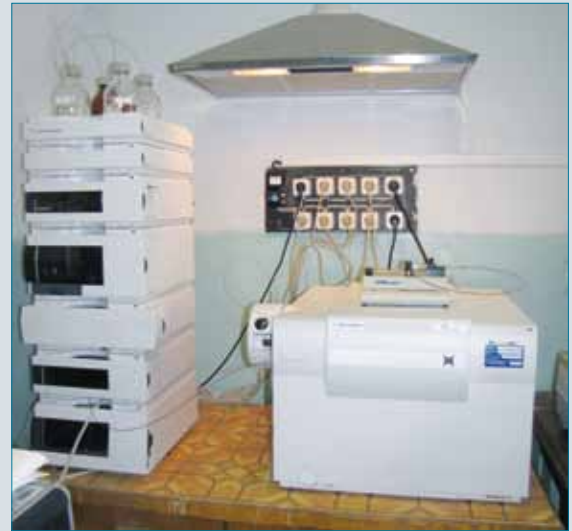
High efficient liquid chromatograph Agilent 1200, with detector of ion trap type ESI-MS Agilent 6330
